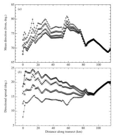
FIGURE 14. Predicted variations of (a)  $\bar{\theta}$  and (b)  $\sigma_{\theta}$  across the shelf for six values of the cutoff parameter  $(k/l)_{\text{max}}$ : --, 5;  $\diamondsuit$ , 4; ×, 3;  $\triangle$ , 2; +, 1; ···, 0.5 (i.e. no Bragg scattering).
