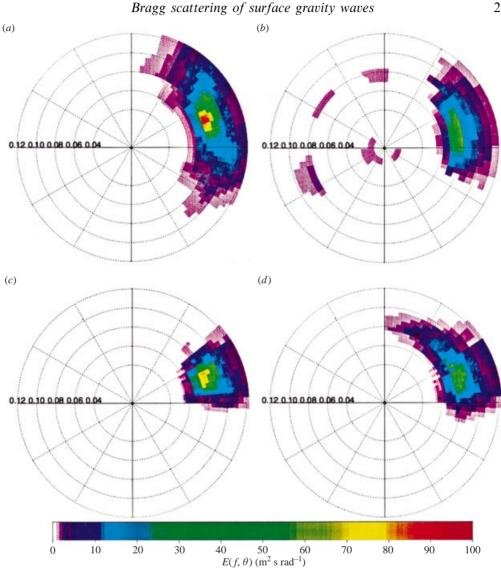
FIGURE 13. Observed wave spectra in (a) 49 and (b) 8 m depth, and predicted wave spectra in 8 m depth, (c) without Bragg scattering and (d) with Bragg scattering, based on the bottom spectrum The function of the second se
