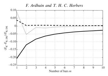
FIGURE 7. Relative differences between the reflected energy predicted by the stochastic theory (equation (3.8)) and the spectral form (equation (3.12), replacing  $\kappa_{\text{DH}}$  by  $\kappa_{\text{DK}}$ ) of Dalrymple and Kirby's theory, as a function of the number of bars *m*. All other parameters are the same as in figure 6. The incident wave spectrum is shown in figure 6.
