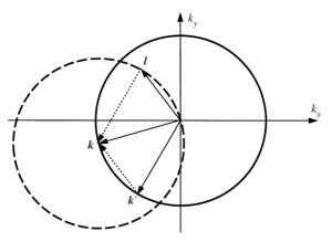
FIGURE 1. Geometric properties of wavenumbers satisfying the resonance condition. The interaction between a surface wave with wavenumber k' and a bottom component with wavenumber l excites a surface wave with the sum wavenumber k = k' + l. For fixed k, the resonant k' and l lie on the solid and dashed circles, respectively.
