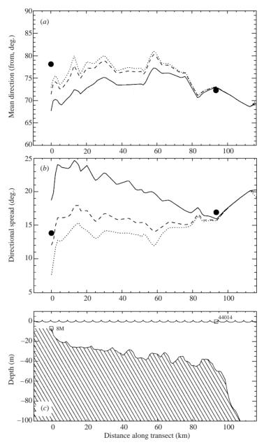
FIGURE 12. Measured ( $\bullet$ ) and predicted (—, with Bragg scattering using  $F_1^B(I)$ ; ---, with Bragg scattering using  $F_2^B(I)$ ; ..., without Bragg scattering) variations of (a)  $\bar{\theta}$  and (b)  $\sigma_{\theta}$  at the peak frequency  $f_p$ . Results are shown for 20 October 2000, at 21:00 GMT, along a cross-shelf transect (c) extending from the 8 m depth array to deep water offshore of NDBC buoy 44014. A maximum value of k/l = 5 was used in the scattering calculations.
