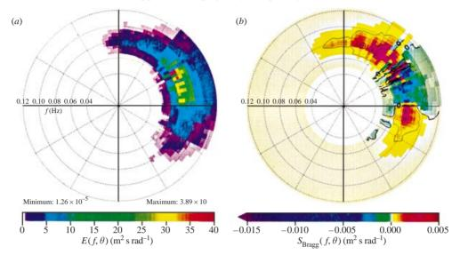
FIGURE 11. (a) Predicted wave spectrum E in region  $S_1$  (figure 8) and (b) corresponding Bragg scattering source term  $S_{\text{Bragg}}$ , based on bottom spectrum  $F_1^B$ . Contours in (b) are solid for positive values (yellow to red colour shades), solid and thick for zero, and dashed for negative values (green to blue colour shades).  $H_s = 0.92 \text{ m}$ ;  $f_p = 0.078 \text{ Hz}$ ; mean direction at  $f_p = 69.5^\circ$ ; spread at  $f_p = 24.00^\circ$ .
